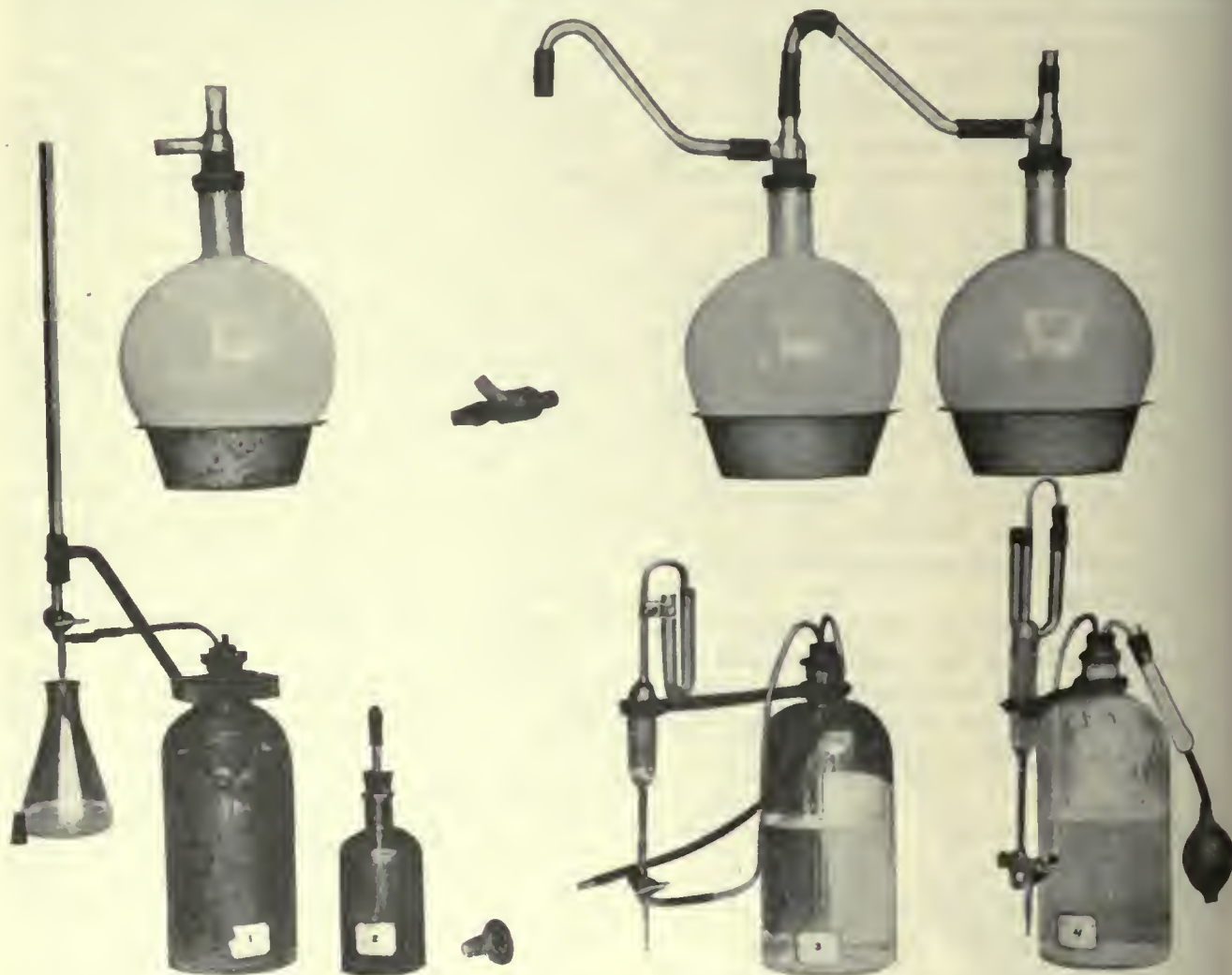
FIG. 68. APPARATUS EMPLOYED FOR CARBON DIOXID DETERMINATIONS
